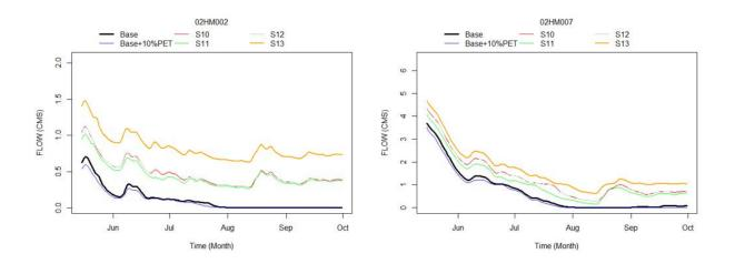
Figure 35. Simulated flow rates at hydrometric stations located along the **Napanee River**, during the June to October 2016 time interval, for the **second set of reservoir evaluation scenarios**.
