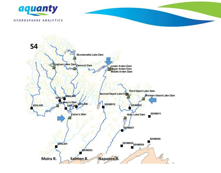
Figure 28. Location (blue arrows) of the reservoirs/dams active for evaluation **scenario 4** in the Moira, Salmon, and Napanee River systems.
