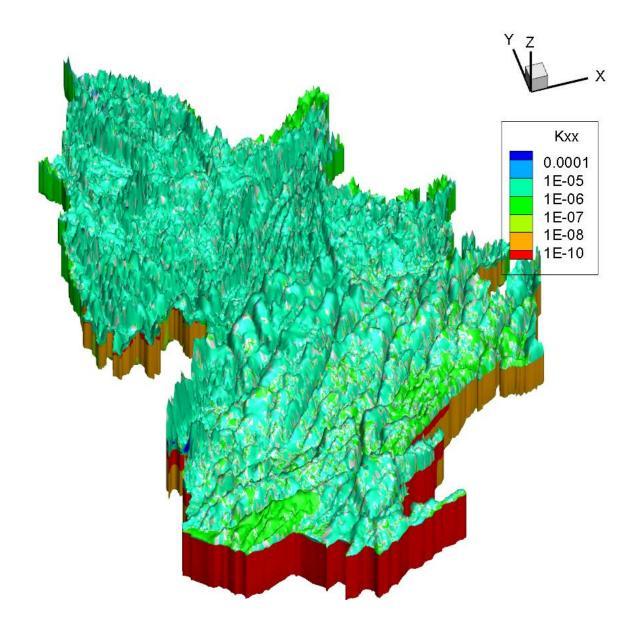
Figure 15. Spatially varying hydraulic conductivity field in the Quinte HGS model.
