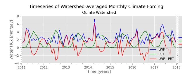
Figure 21. Temporal variability of watershed-average liquid water forcing (LWF) and potential evapotranspiration (PET), used as climate forcing data for the model, over the 2011 to 2018 simulation interval. Also shown (in red) is the LWF – PET as a proxy for water deficit. The vertical bar on the right-hand side shows the long-term average of each variable.
