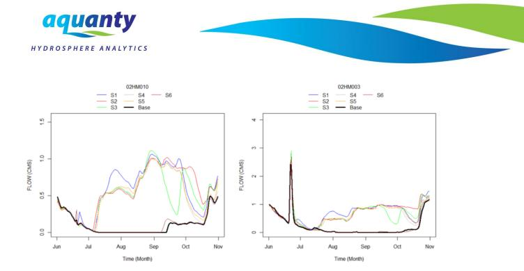
Figure 31. Simulated flow rates at hydrometric stations located along the **Salmon River**, during the June to November 2016 time interval, for the **first set of reservoir evaluation scenarios**.
