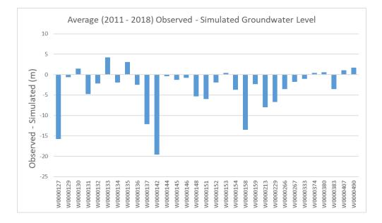
Figure 26. Difference in long term (2011 – 2018) daily average observed and simulated groundwater levels in the 31 PGMN wells used to evaluate model performance.
