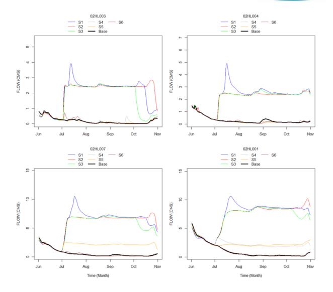
Figure 30. Simulated flow rates at hydrometric stations located along the **Moira River**, during the June to November 2016 time interval, for the **first set of reservoir evaluation scenarios**.
