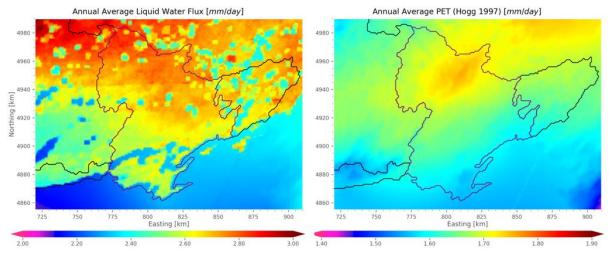
Figure 19. (Left panel) 2011 to 2018 average spatial distribution of liquid water flux (LWF) over the model domain. (Right panel) 2011 – 2018 average spatial distribution of potential evapotranspiration (PET) over the model domain.
