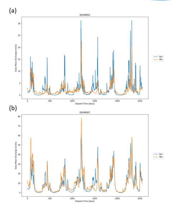
Figure 24. Simulated versus observed surface water flow rates at the hydrometric station with the (a) lowest, and (b) the highest NSE values. Note that Day 0 represents January 1, 2011 and the time series extends to Day 2555, which reflects December 31, 2018.
