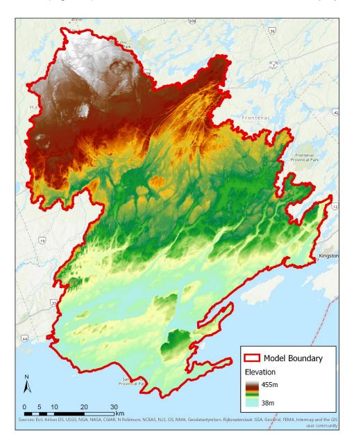
Figure 4: Stitched Ontario Integrated Hydrology DEM, NOAA bathymetry, and inland lake bathymetry from Quinte Conservation. Resolution 30m in UTM 17N.
