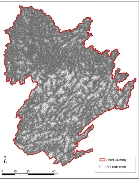
Figure 12: Updated mesh for Quinte. Each mesh sheet contains 73,049 nodes and 143,990 elements.
