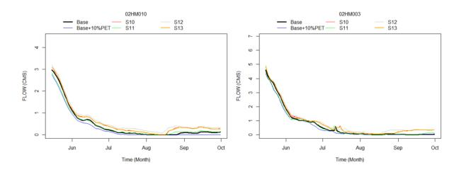
Figure 34. Simulated flow rates at hydrometric stations located along the **Salmon River**, during the June to October 2016 time interval, for the **second set of reservoir evaluation scenarios**.
