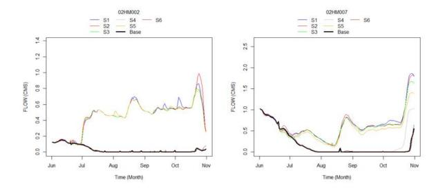
Figure 32. Simulated flow rates at hydrometric stations located along the **Napanee River**, during the June to November 2016 time interval, for the **first set of reservoir evaluation scenarios**.
