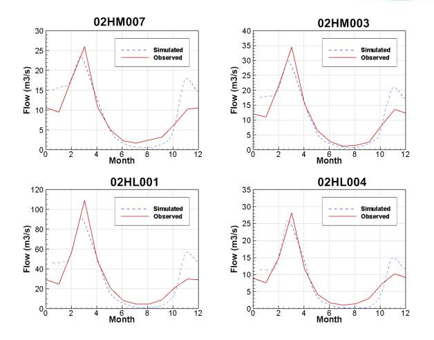
Figure 18. Representative monthly normal hydrographs showing simulated vs. observed flow conditions at four Water Survey of Canada Hydrometric Stations. Note that in total there are 16 hydrometric stations configured in the HGS model.
